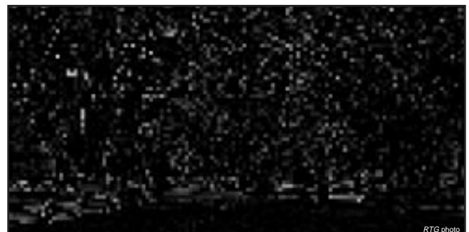
The absolute values of the differences between (b) and (c) correspond to the errors in each pixel in the rendering in (b). The r.m.s. of these errors is a measure of the image quality, and note that it can be computed without displaying any of the images.
